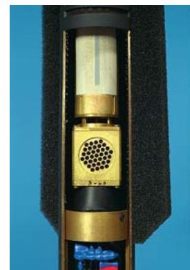
The middle system (M-signal) combines high attenuation of lateral sound incidence, similar to a hypercardioid characteristic (which is about 10 dB), with the large front-to back ratio of the super-cardioid characteristic.
