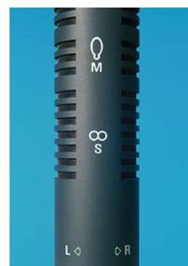
The side system (S-signal) consists of two single capsules arranged back to back, closely behind the interference tube (M-signal) capsule. Arrows engraved on the microphone housing show their orientation.
