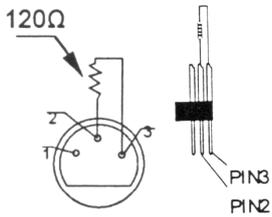
A DMX terminator is recommended for installations where the DMX cable has to run a long distance or is in an electrically noisy environment (e.g. discos). The terminator prevents corruption of the digital control signal by electrical noise. The DMX terminator is simply an XLR plug with a 120Ω resistor between pins 2 and 3, which is then plugged into the XLR output socket of the last device in the chain. Please see illustrations.
